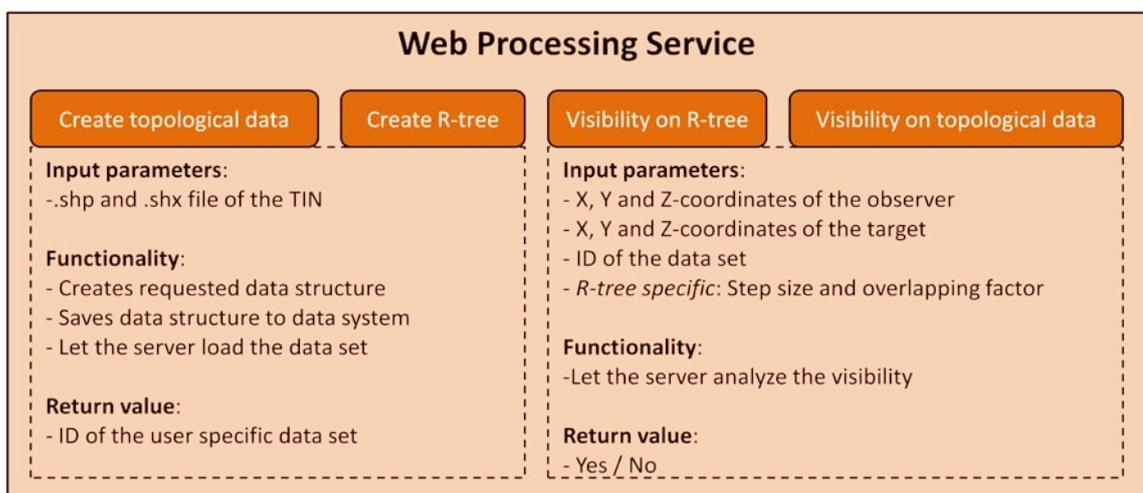
**Fig. 28:** The four WPS processes in detail.
