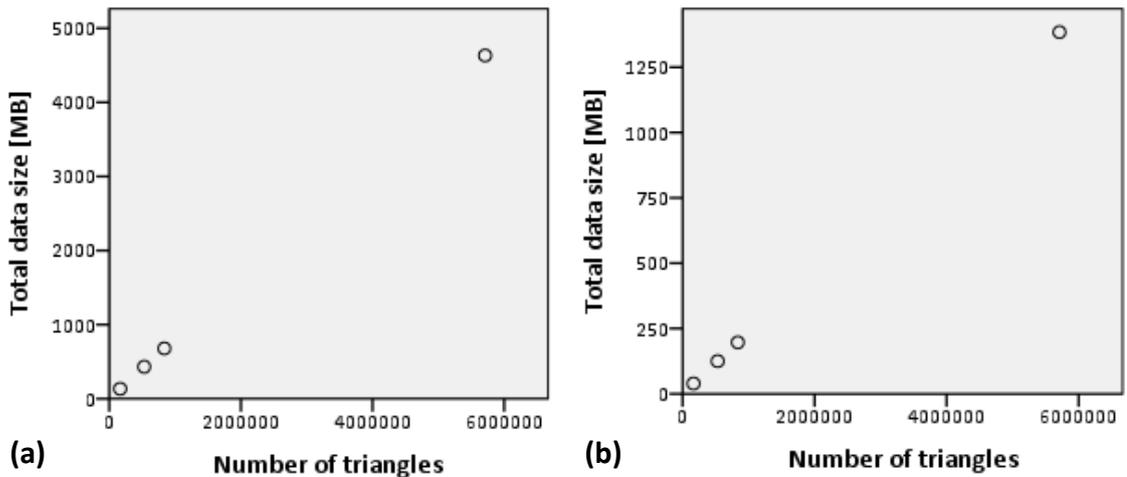
**Fig. 31:** Scatter plots between the number of triangles and the total data size of the R-tree (a) and the topological data structure (b).
