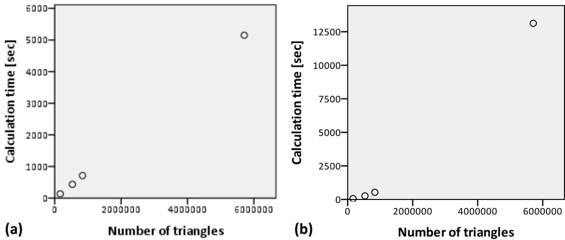
**Fig. 30:** Scatter plots between the number of triangles and the calculation time for the R-tree (a) and the topological data structure (b).
