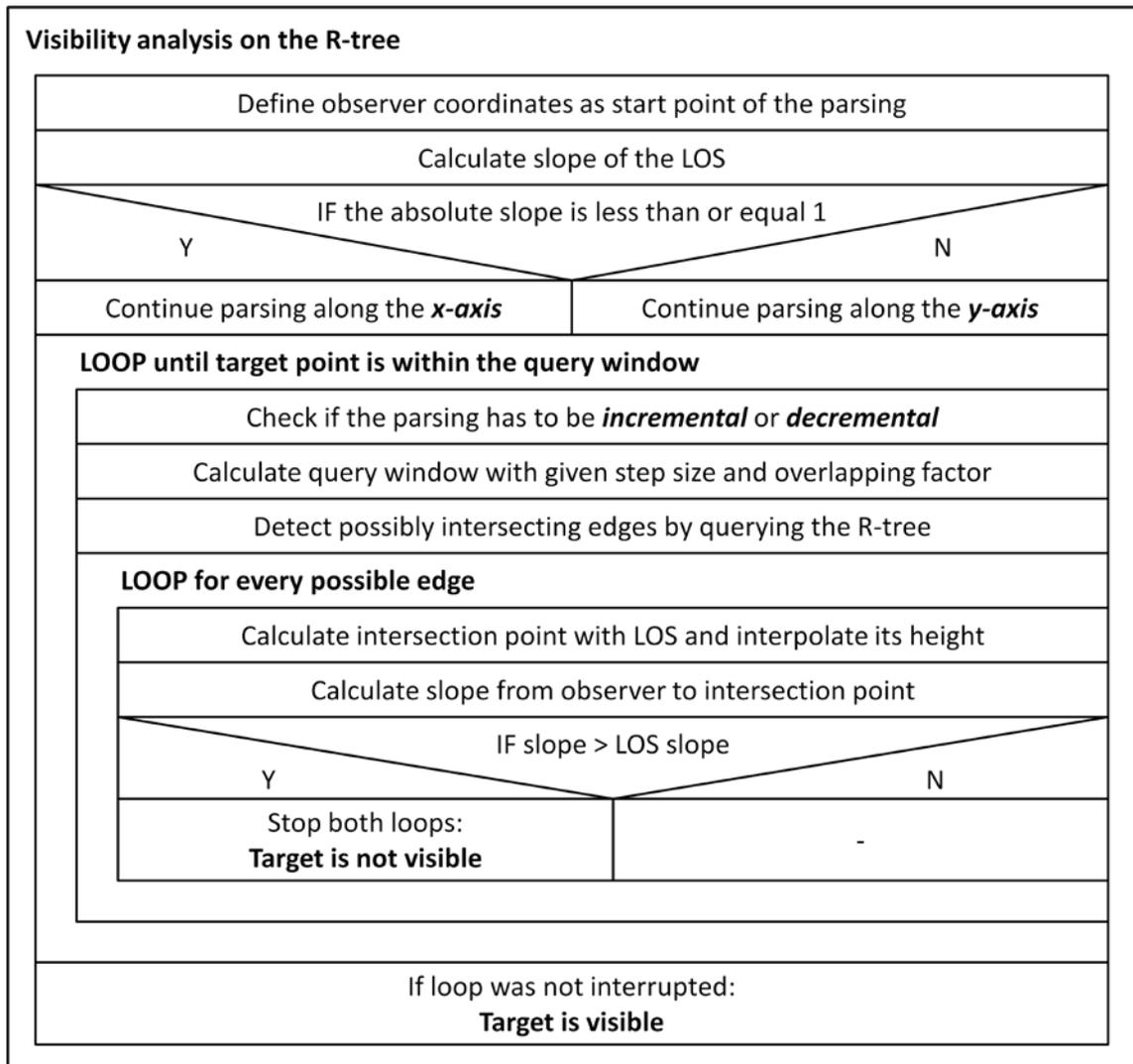
**Fig. 21:** The logic of the visibility algorithm.
