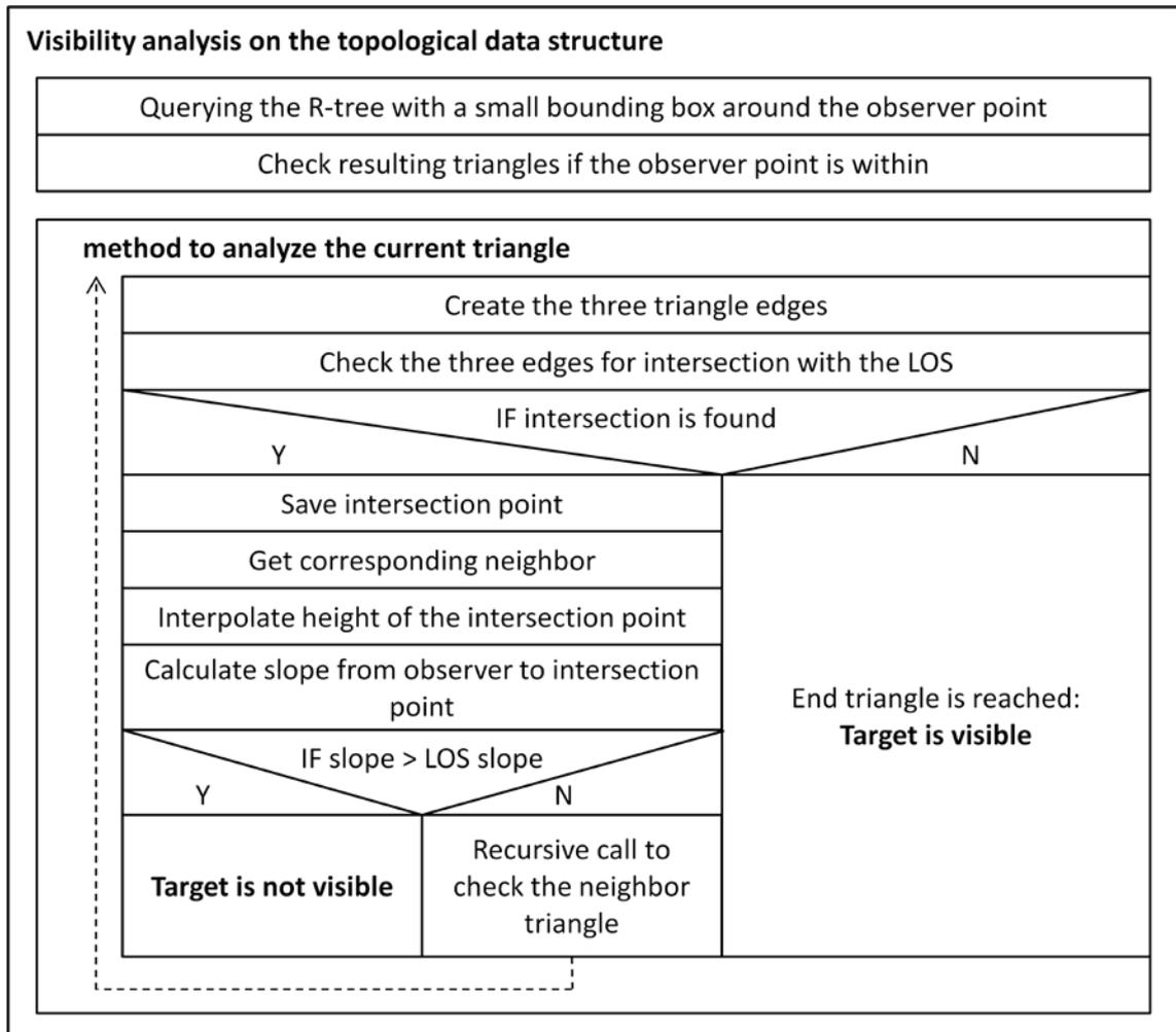
**Fig. 26:** The logic to analyze the visibility on the topological data structure.
