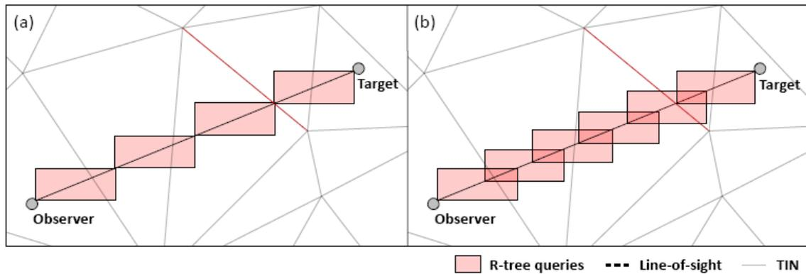
**Fig. 20:** Possibly undetected intersection (red line) with the TIN (a), avoided by overlapping query windows (b).
