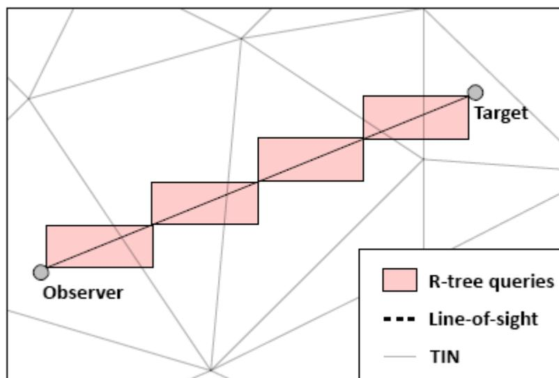
**Fig. 17:** General idea of the visibility analysis using the R-tree
