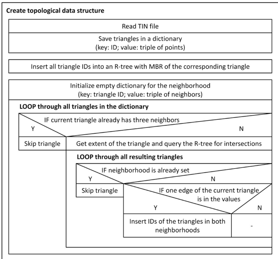
**Fig. 25:** The logic to create the topological data structure.
