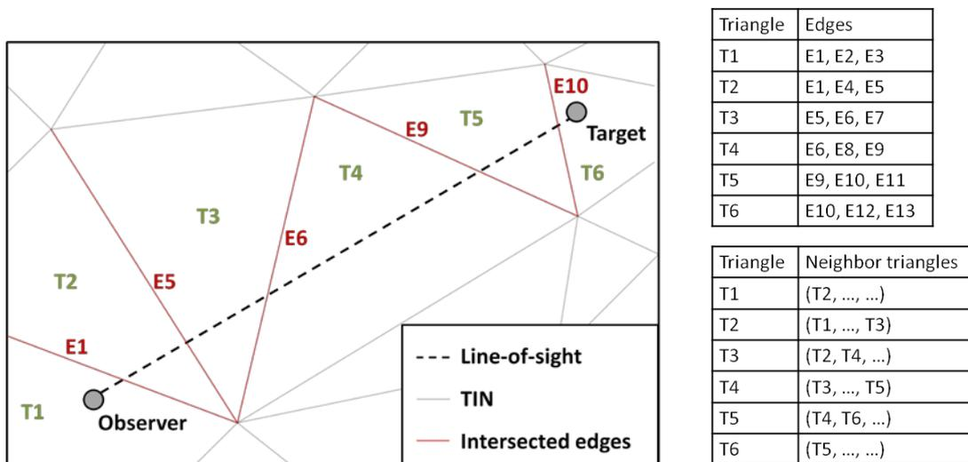
**Fig. 24:** General idea of the visibility analysis using a topological data structure.
