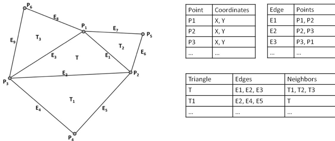
**Fig. 22:** Four triangles with their points and edges and the corresponding topological data structure.
