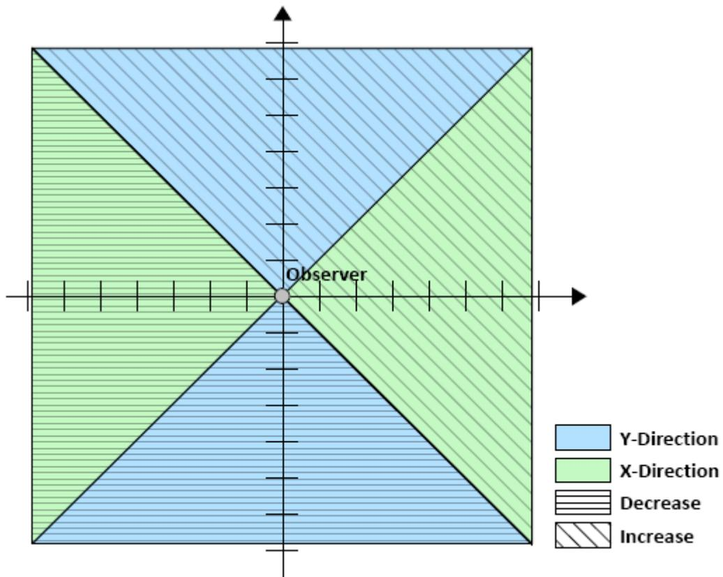
**Fig. 19:** The blue and green zones show the different parsing directions according to the slope of conceived lines-of-sight. The different line directions symbolize the zones in which the direction increases or decreases.
