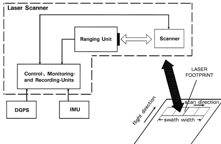
**Fig. 2:** A typical ALS system. (Wehr and Lohr, 1999:69)
