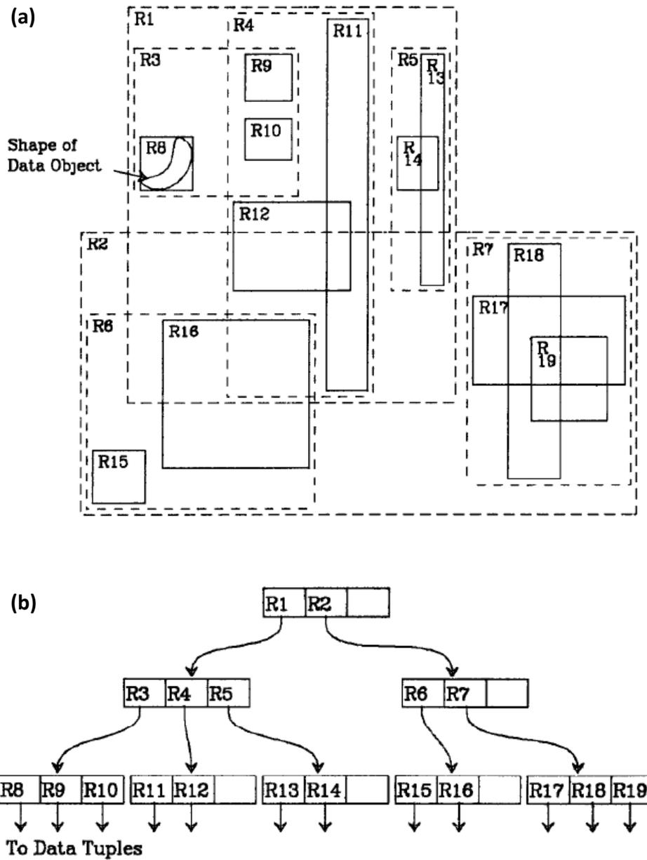
**Fig. 16:** (a) An example of nested minimally bounding rectangles (solid and dashed lines). R8 shows a sample data. (b) The corresponding R-tree data structure.
