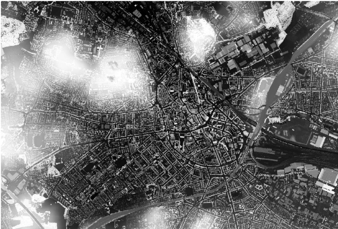
**Fig. 12:** Digital surface model (DSM) of Osnabrück (high elevations: bright; low elevations: dark).
