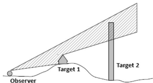
**Fig. 3:** The field of view of an observer. Target 1 is fully and target 2 is partially visible.
