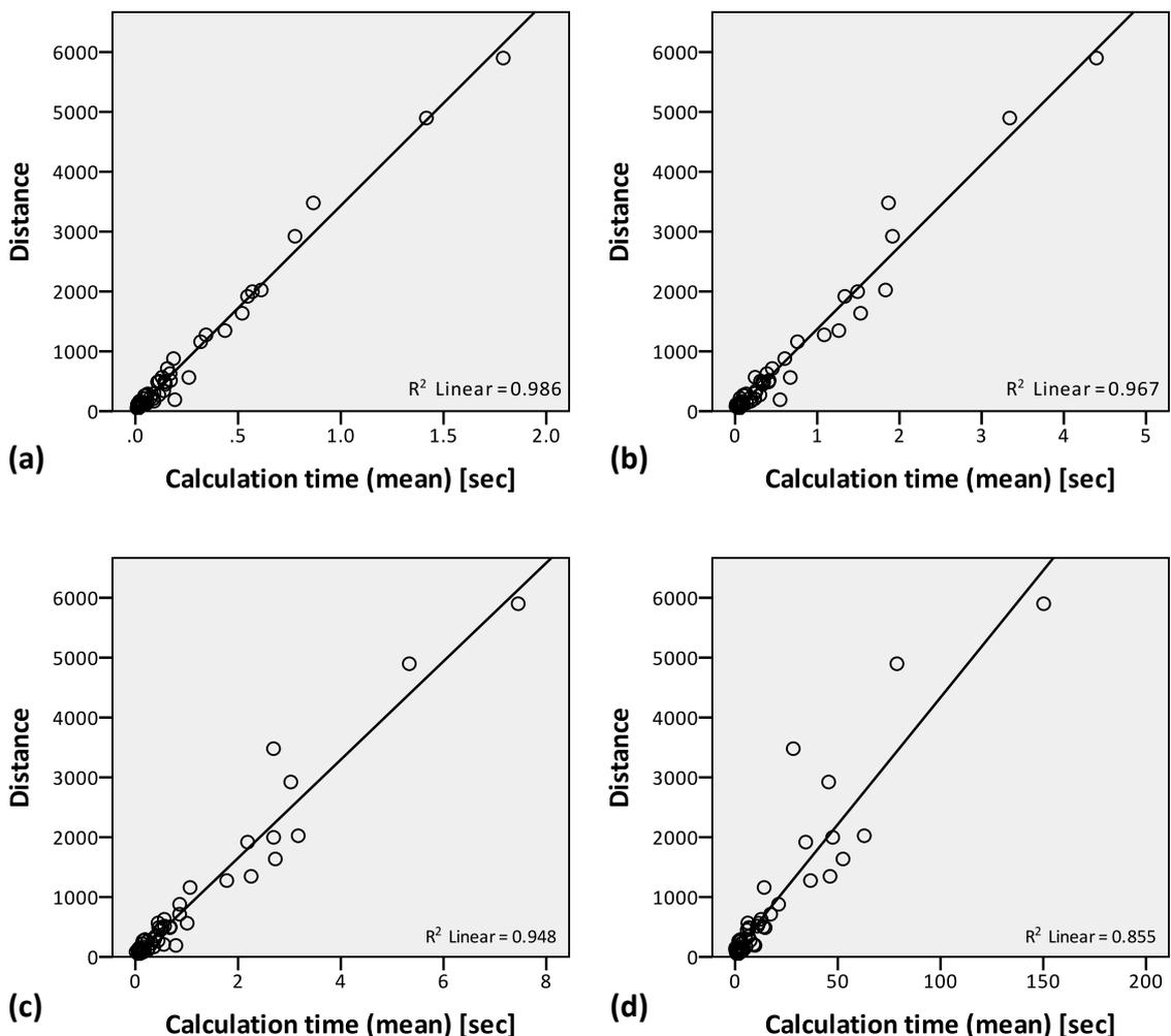
**Fig. 32:** Scatter plots between the distance from the observer to the target and the mean calculation time of the R-tree on TIN15 (a), TIN10 (b), TIN8 (c) and TIN2 (d).
