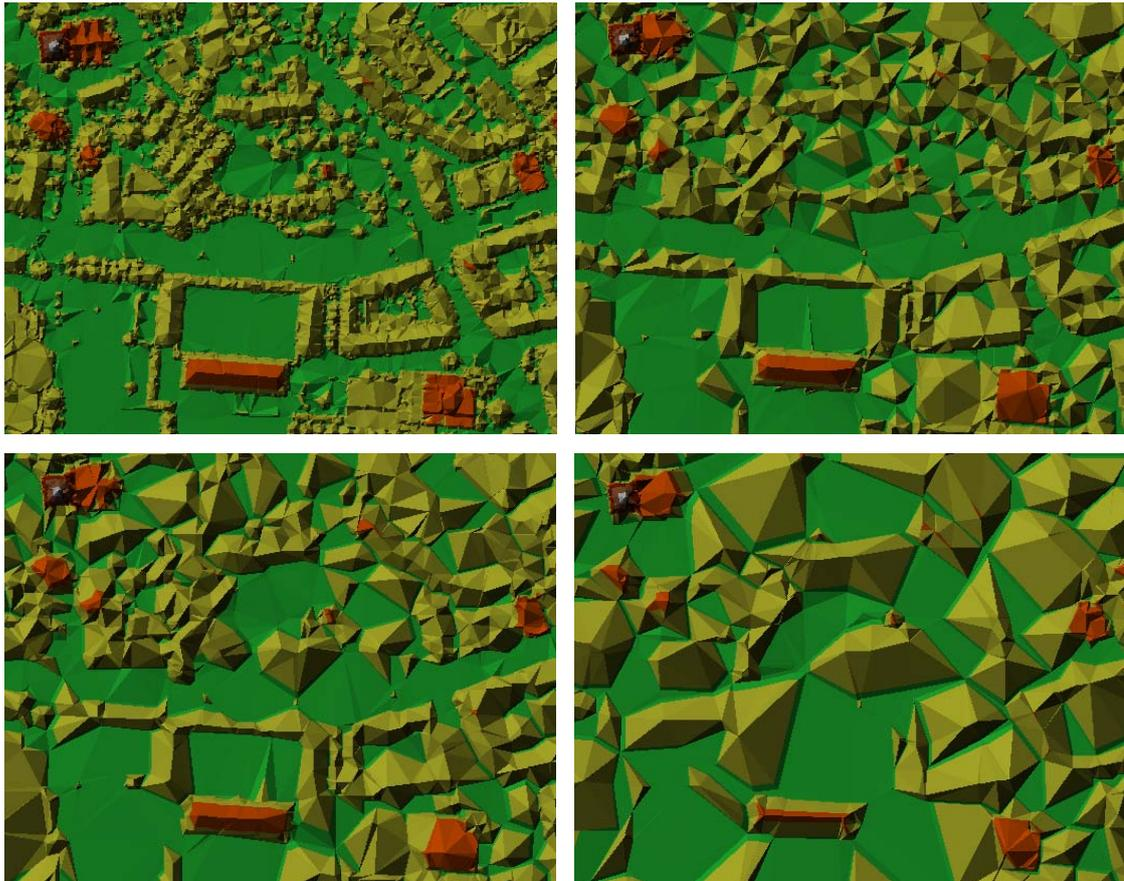
**Fig. 15:** The four available TINs of a part of the city center of Osnabrück. Top left: TIN2;
