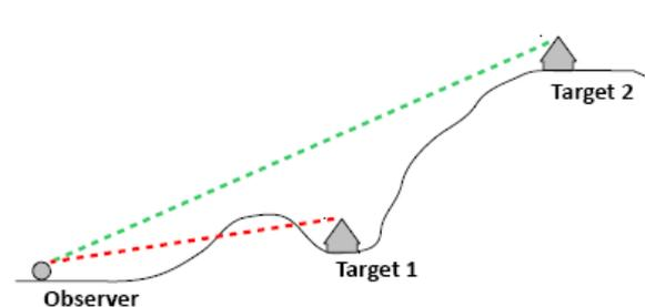
**Fig. 4:** The direct lines (LOS) between an observer and two targets. Target 2 is visible while target 1 is hidden behind the terrain.
