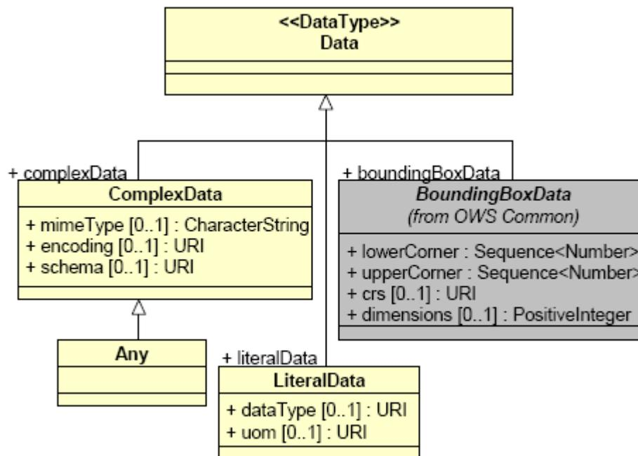
**Fig. 9:** UML diagram of the three different data types of the WPS.
