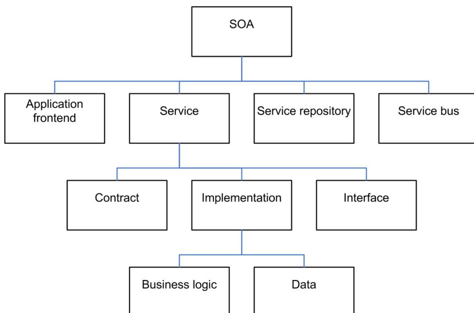
**Fig. 8:** Overview of the components of a SOA. (Krafzig et al., 2004:57)
