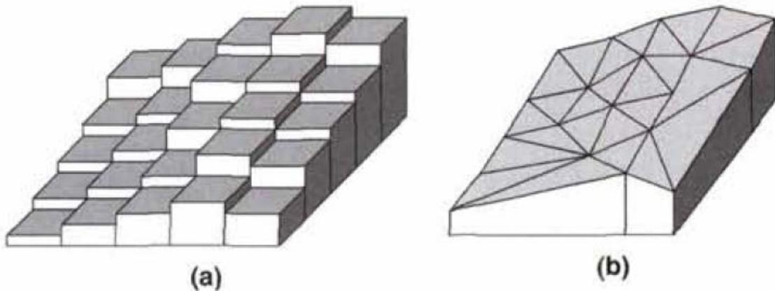
**Fig. 6:** Raster (a) and TIN (b) data models of the same terrain.
