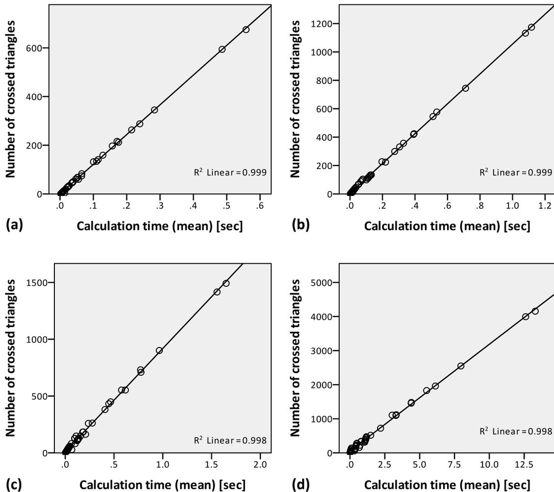
**Fig. 33:** Scatter plots between the number of crossed triangles by the LOS and the mean calculation time of the topological data structure on TIN15 (a), TIN10 (b), TIN8 (c) and TIN2 (d).
